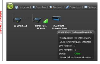
Recognizing the 3633PWM-H using Wireless DMX RDM (Screenshot: CRMX Nova Software)
